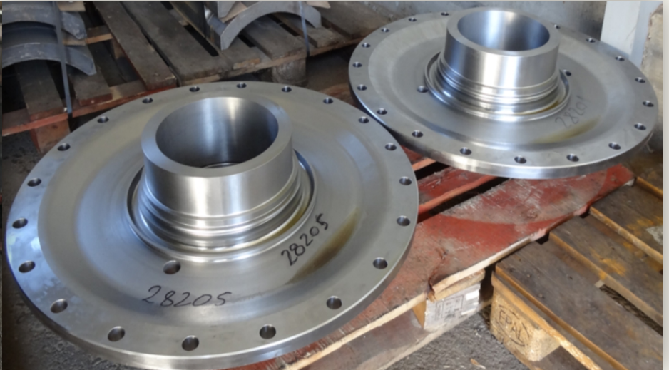
locomotive bogie hubs 250 kg, material: GE300
