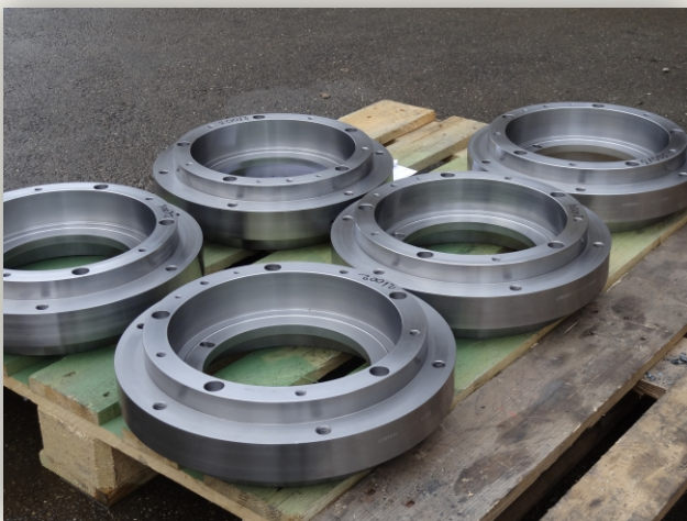
Bearing bushings 45 kg, material: 34CrNiAl7-10
