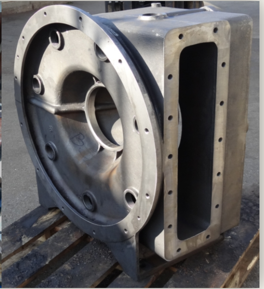
turbine housing 380 kg, material: EN-GJL-200
