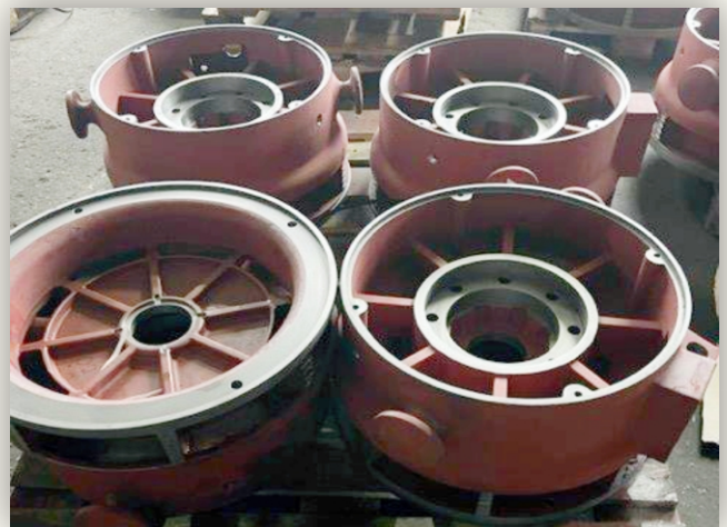
Pump sleeve bodies 185 kg, material: EN-GJL-250
