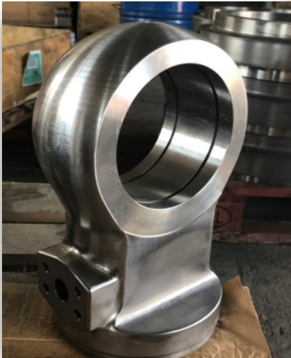
hidraulic cylinder head 15 kg, material: S355 J2
