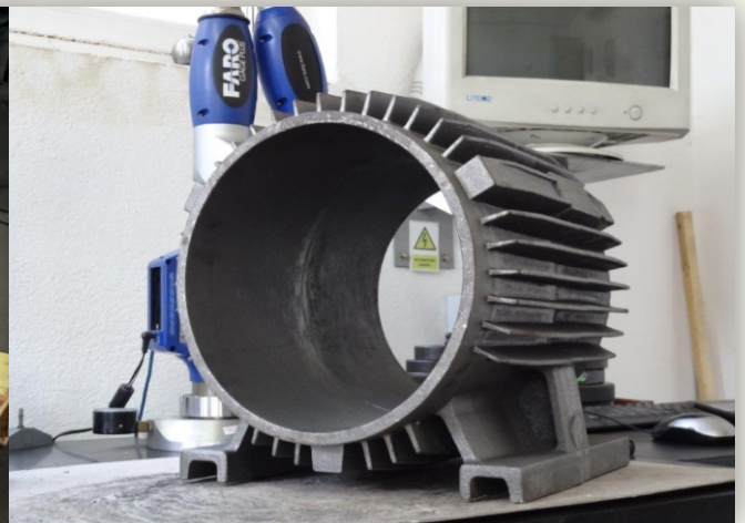
electric motor housing 35 kg, material: EN-GJL-250
