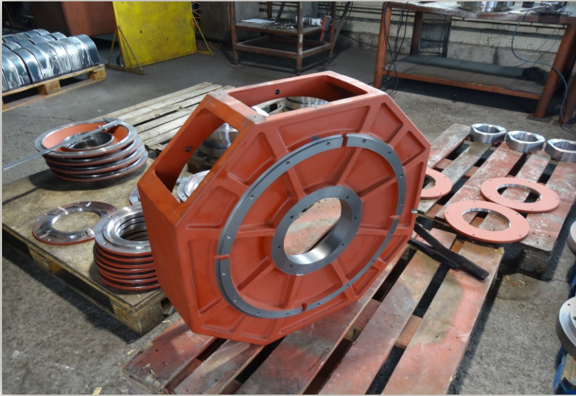
electric generator shield 200 kg, material: EN-GJS-400-15
